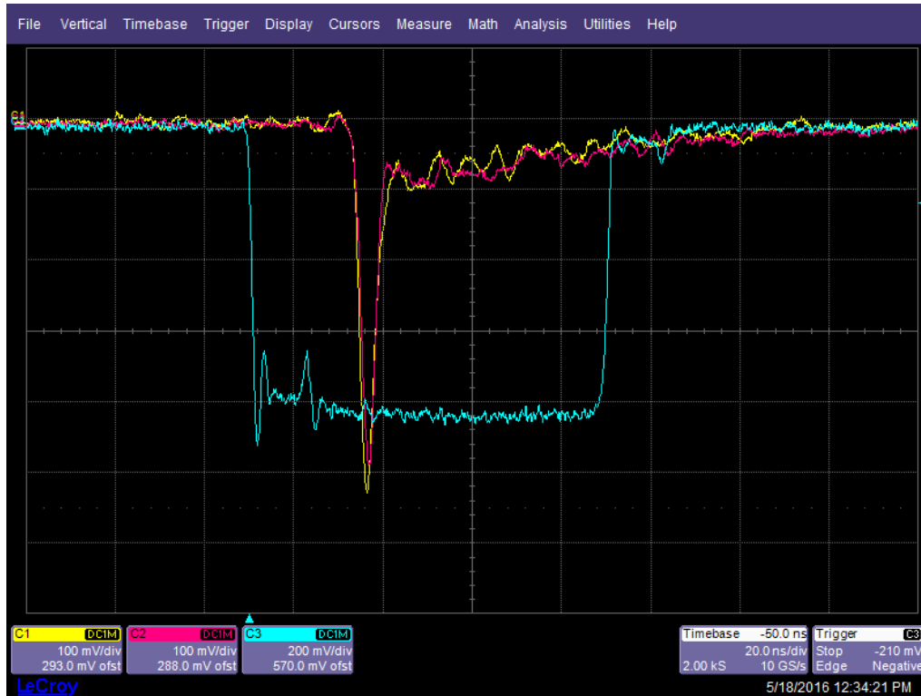
Figure 6.5: Trigger signal (blue) and analog signal from the two sensor boards (yellow and pink)
