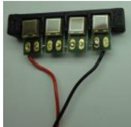
Figure 5.2: serial connection of (KETEK) SiPMs
