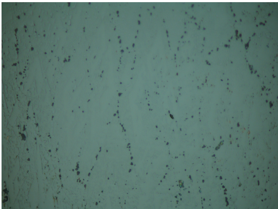
Fig. 45. A picture of sample S6 (taken under the light microscope (50x). Dark precipitate of \text{HfO}_2 is observed in the smaller amount than in the previous samples (Fig. 44) which is believed to be a result of the oxygen dissolution in pure hafnium which is one of the phase present in this sample
