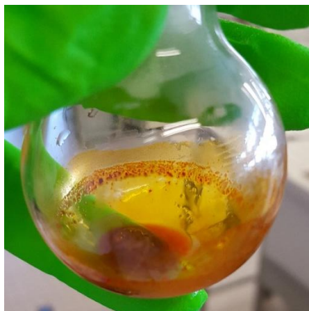
Figure 33: Round bottomed flask during preparation of CAT-CAL-lipo. Aggregation on the side wall is clearly visible.
