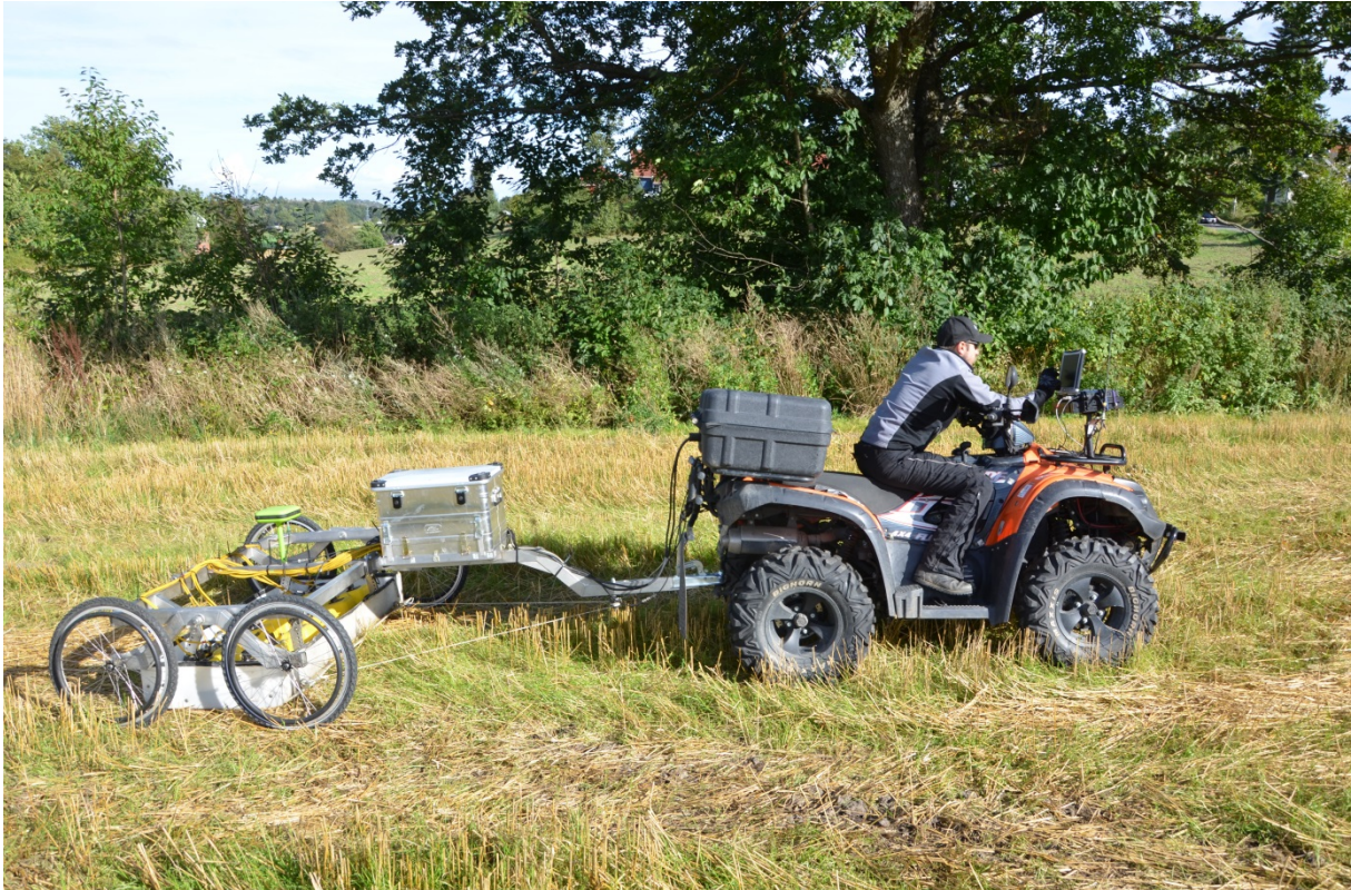
Fig. 1.8 State-of-the-art motorised multichannel GPR array pulled by an ATV
