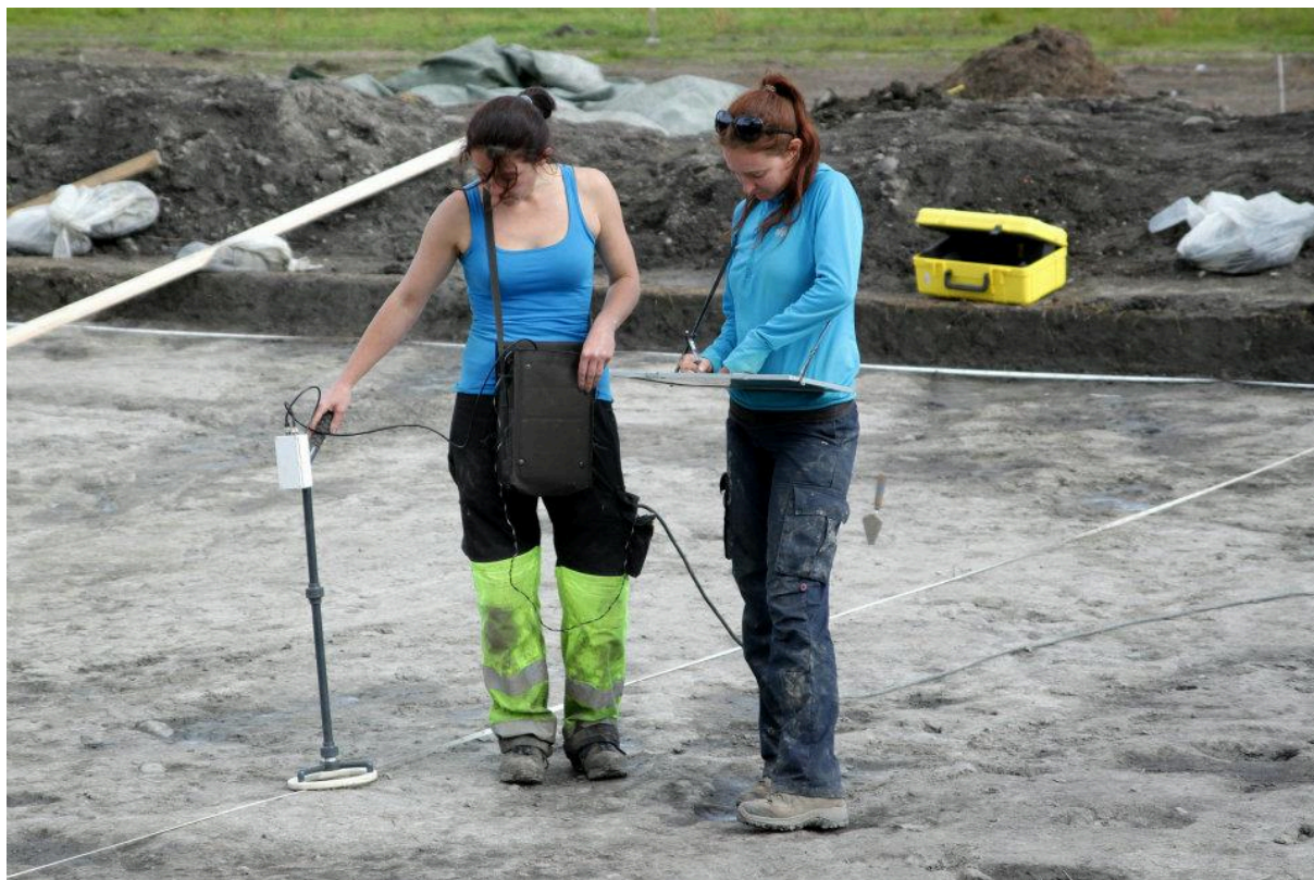
Fig. 5.9 In-situ volume susceptibility measurements in trench 1 after removal of top soil using a Bartington susceptibility meter and a MS2D probe
