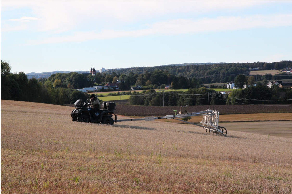
Fig. 1.5 Motorised magnetic multi fluxgate gradiometer array pulled by an all-terrain-vehicle (ATV)
