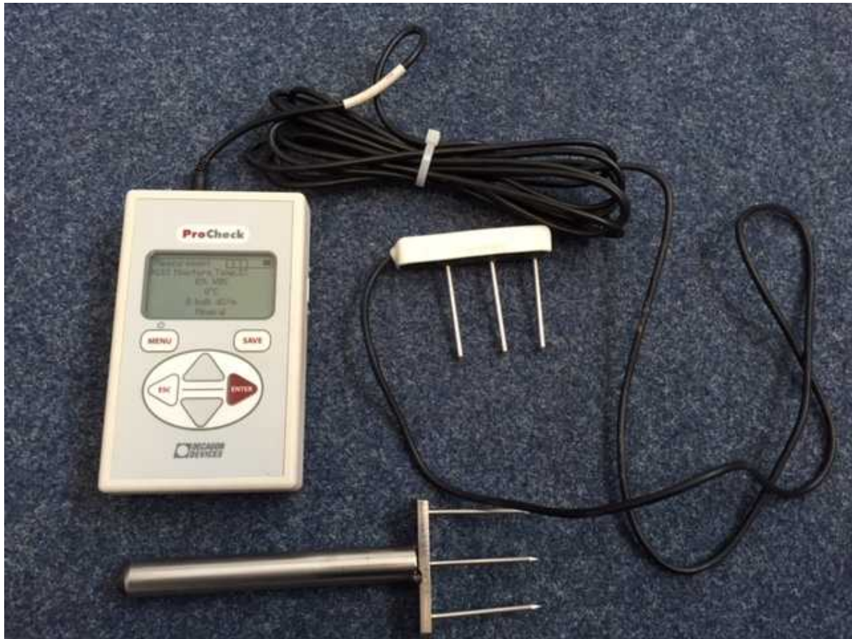
Fig. 6.4 Moisture sensor with custom-made steel piercer
