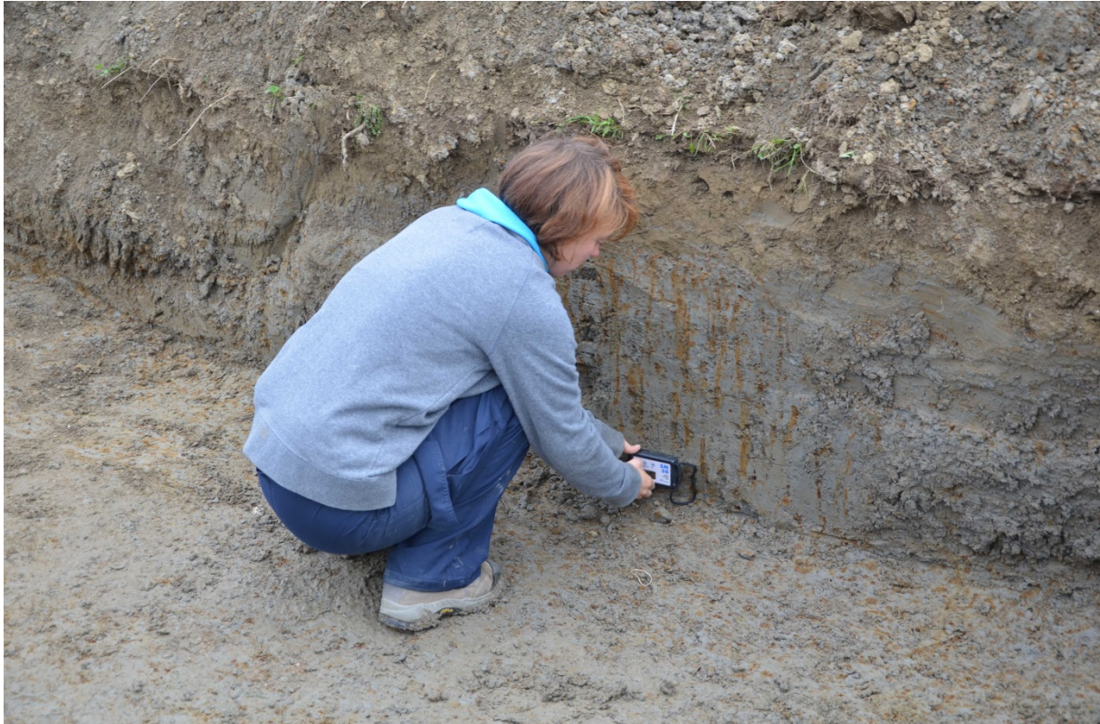
Fig. 6.3 The hand-held kappa meter SM-30 used to measure volume MS in the field
