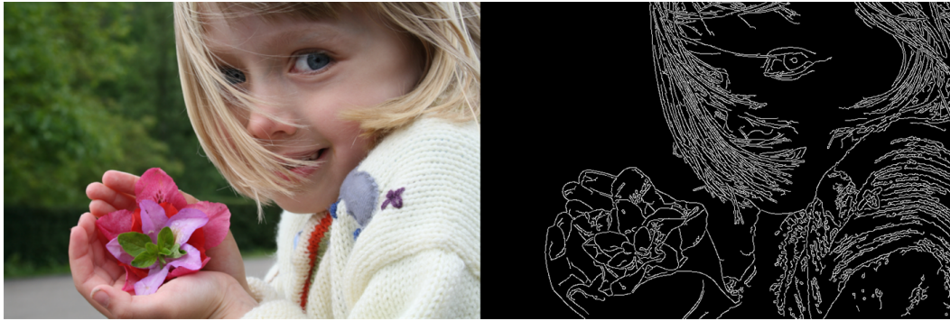
Figure 5.2: Edge detection using the Canny algorithm 1
