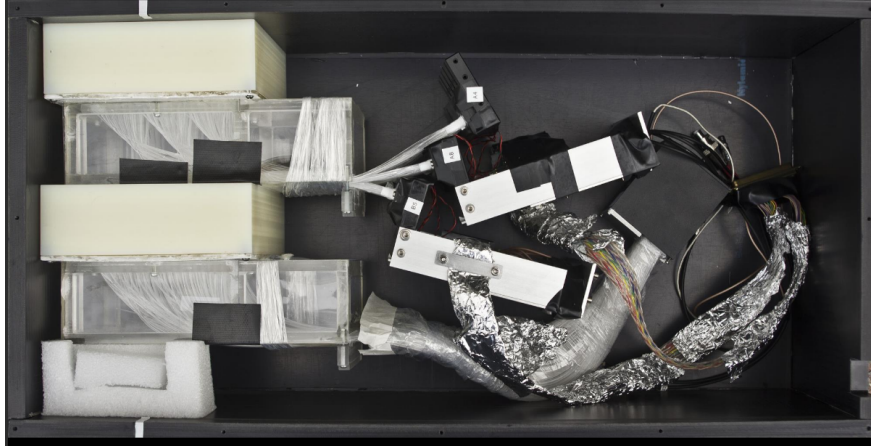
FIGURE 2.6: The box with 2 detectors placed next to each other to be tested in one run. (Photograph by W.H.Trzaska)
