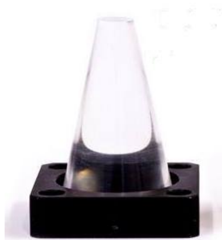
FIGURE 3.9: A plastic light guide made out of acrylic glass with holder.
