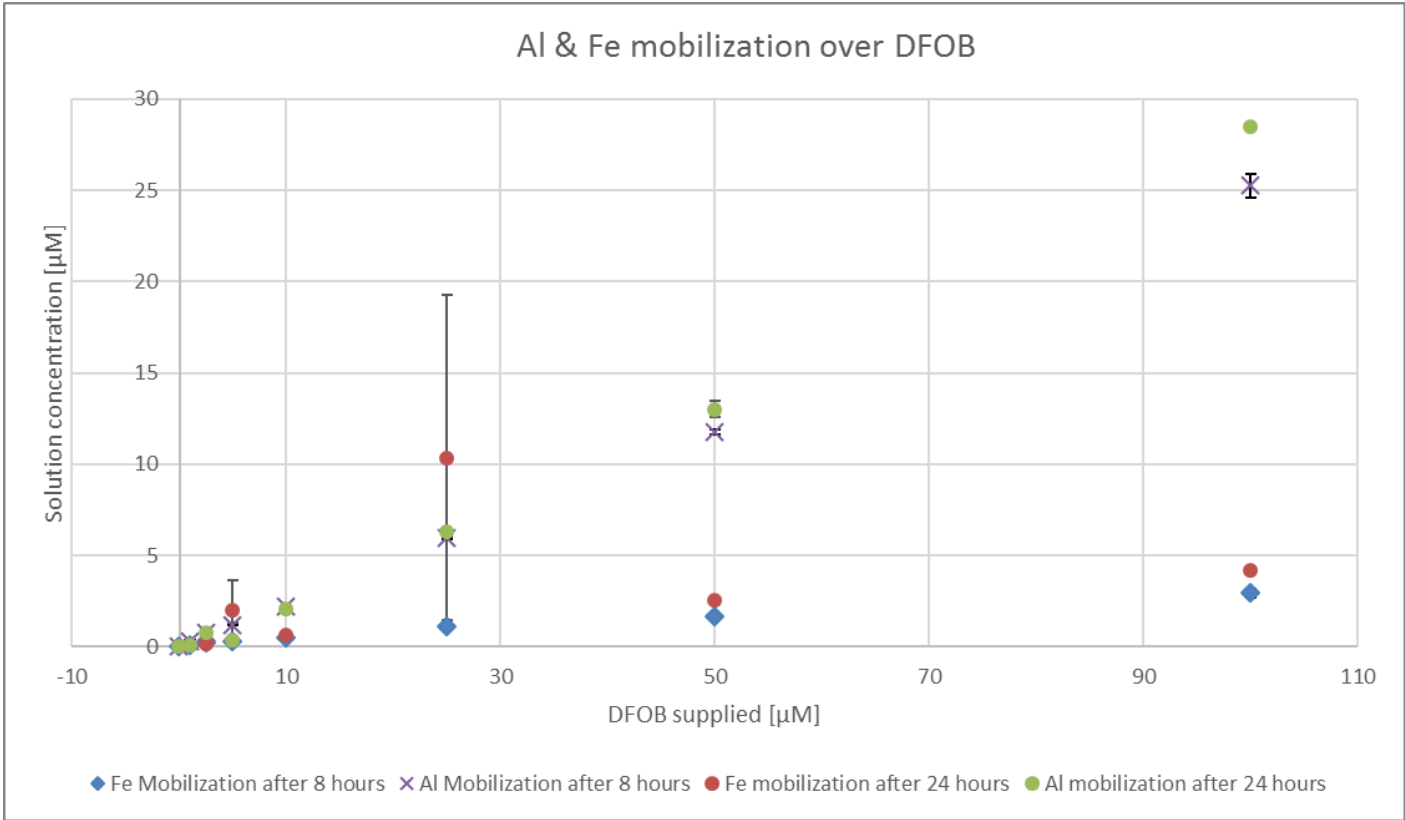
SI Figure 17 Results Interaction of 0-100 \mu\text{M} DFOB 8h & 24h; 10mM \text{CaCl}_2 0.2g/L Bronopol; Values presented are corrected for the mean blank concentrations; n=2; SSR 1:5; Xeraco soil
