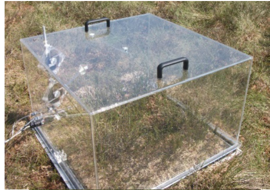
Figure 14: Transparent Closed Dynamic Chamber
