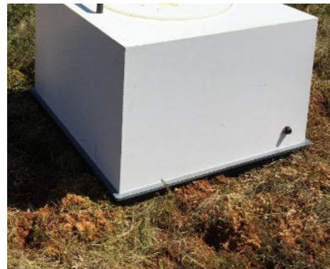
Figure 15: Opaque Closed Dynamic Chamber
