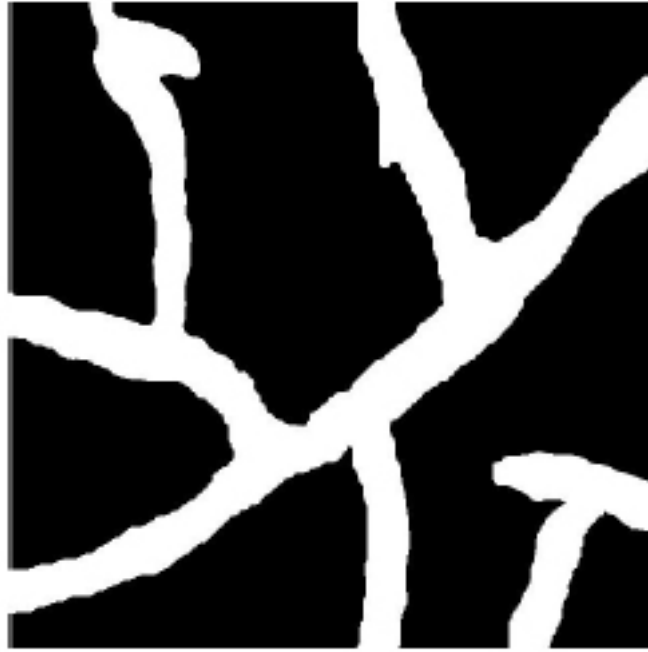
Figure 6: Pore structure of the Vycor glass (reproduced from (19)).
