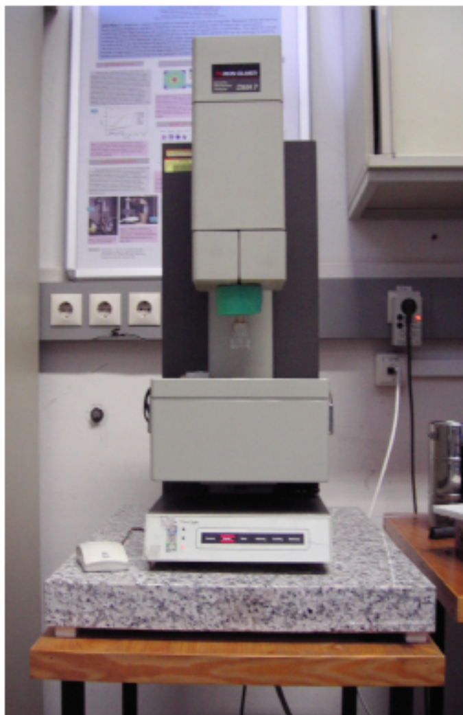
Figure 2. The Perkin Elmer series 7 dynamic mechanical analyser (reproduced from (81)).
