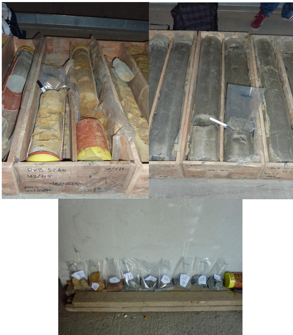
Figure 6: Core boxes with sample positions (above) and sampled material (below) at the MA 29 drilling core storage
