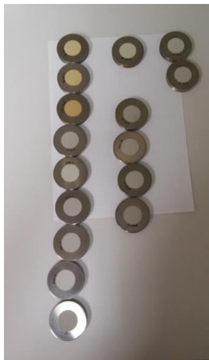
Figure 8: Pressed pellets ready for XRD analysis
