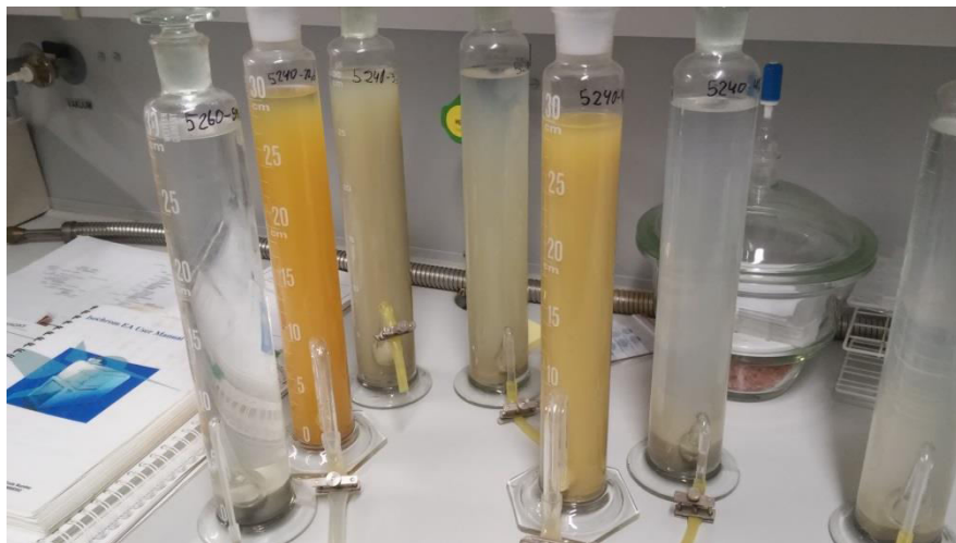
Figure 9: Sedimentation in Atterberg cylinders
