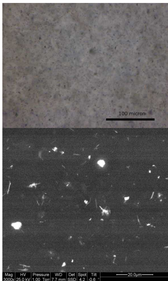
Figure 3 Optical (top) and scanning electron microscopy (bottom) [6] images of JD-2000 filled with \approx 1 wt-% MoS 2 .
