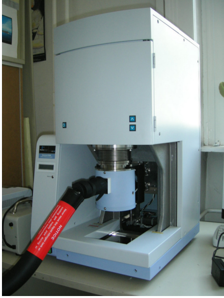
Figure 4.2: Unmodified Perkin Elmer Diamond DMA. An insulated hose connects the liquid nitrogen dewar to the instrument's furnace.
