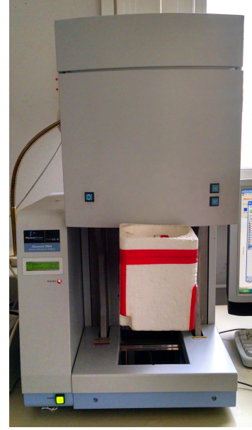
Figure 4.3: Modified Perkin Elmer Diamond DMA. The insulated liquid nitrogen reservoir is mounted directly on the furnace. The top covering of the reservoir was removed and is not shown in the picture.
