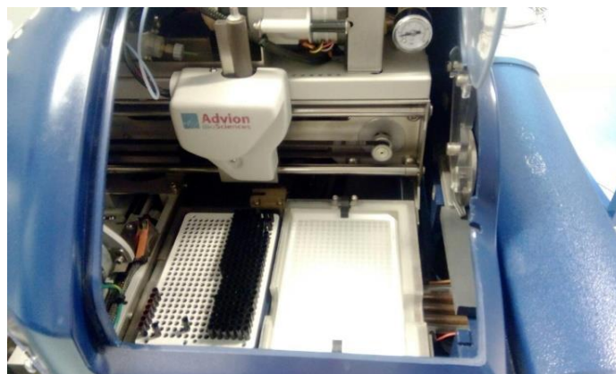
Figure 8. Inner part of the Advion Triversa NanoMate®: On the bottom are tip wrack (left) and 384-well well plate (right). The well plate is positioned on a plate cooler allowing temperatures from 4°C to 25°C. Above is a robotic part of the NanoMate® for sample collection and transport to ESI chip.
