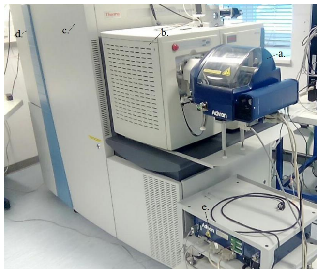
Figure 11. LTQ-Velos™ Hybrid Ion Trap-Orbitrap Mass Spectrometer physically coupled to the ETD module. a) TriVersa NanoMate® Advion, b) LTQ Velos module, c) Orbitrap module, d) ETD system module, e) Interface to link the mass spectrometer, the NanoMate® and the computer together.
