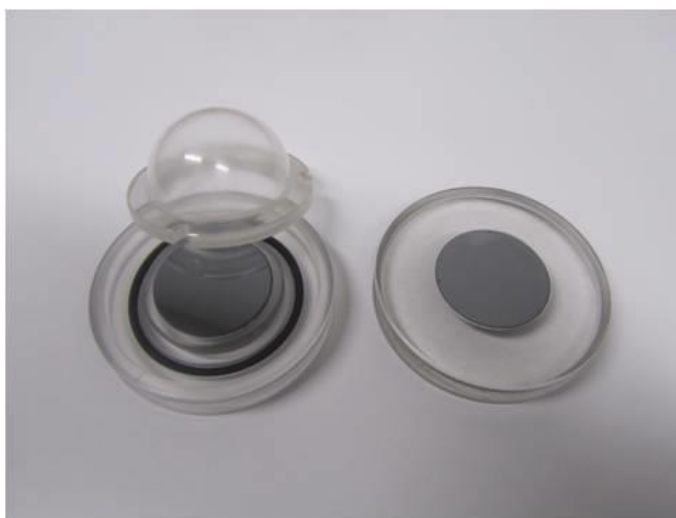
Fig.7. The sample holders used for X-ray powder diffraction (XRD) study.
