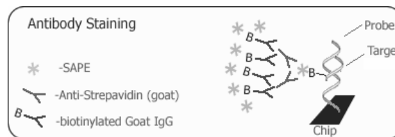
Figure 19: Schematic representation of staining of Hybridized DNA. The affymetrix version uses an anti-Streptavidin (goat) biotin conjugated antibody; however Goat IgG is added in order to avoid non specific interactions.
