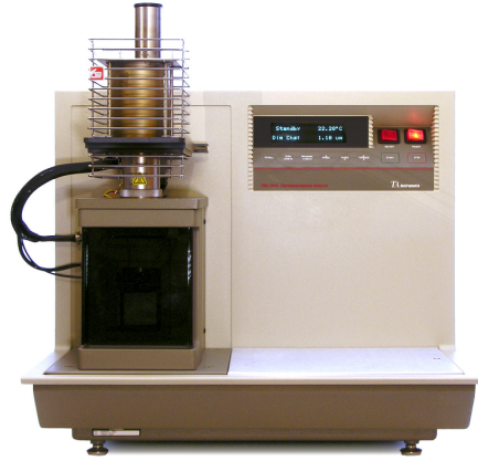
Figure 31: TA 2940 Thermomechanical Analyzer[105]
