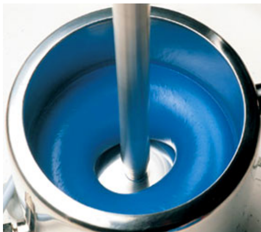
Figure 27: The doughnut effect during the slurry preparations[90]
