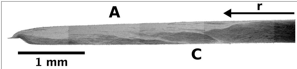
Figure III-1.: Combined SEM images of a cross section of the HPT deformed Co 3 Ti-I disc. The images are acquired by the BSE detector using a high tension of 20 kV. The bright areas in the image correspond to amorphous regions whereas the dark areas are still crystalline. Amorphous regions are located at one half of the sample towards the surface indicated with (A). The other sample surface revealing more crystalline regions is marked with (C). The radial direction of the disc is indicated with an arrow (r). Just one half of a cross section is shown in the image.
