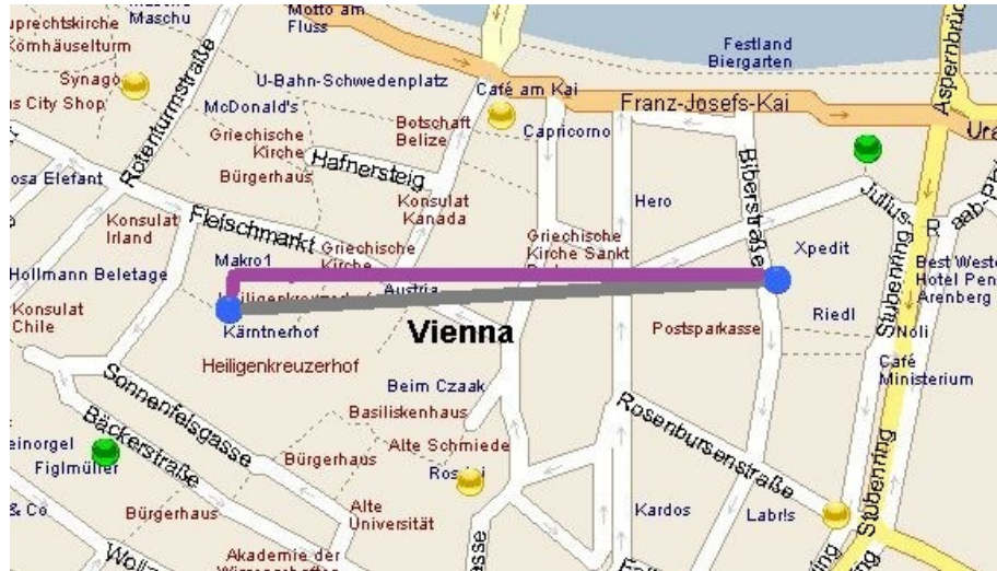
Figure 7. Example of the C-C Euclid and C-C Manhattan approaches
