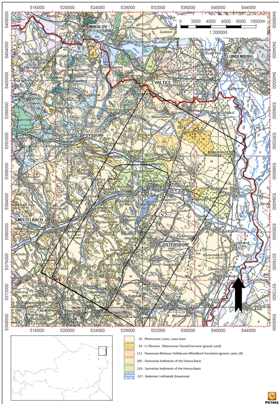
Fig. 1: Geological map with place names of the investigated area. The black rectangle (28 km x 15 km) marks the border of the seismic volume. The polygon inside represents the border of the mapped flysch horizon. MGI Austria GK M34 coordinate system including a false easting of 500,000.
