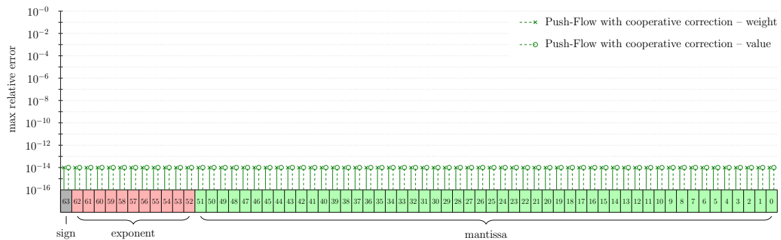
Figure 4.11: PFCC: Maximum relative error over all nodes induced by single bit-flips on different positions in floating-point variables holding the value or weight (maximum over 100 runs each point, Python Discrete Event Simulator (Appendix A.3), 32 nodes, hypercube communication topology, \varepsilon = 10^{-14} )
