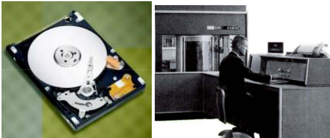
Figure 3.6: Nowadays it is easy to get a 1 Tb hard disk, left picture. But just a few decades ago a computer as big as a room could only store 40 Mb, right picture. Pictures taken from [80].
