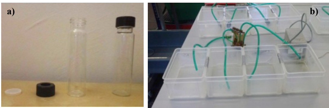
Figure 16 (a) Glass-vials used for respiration measurements. 16 (b) Aquaria used for acclimatization of Hydropsychidae larvae.
