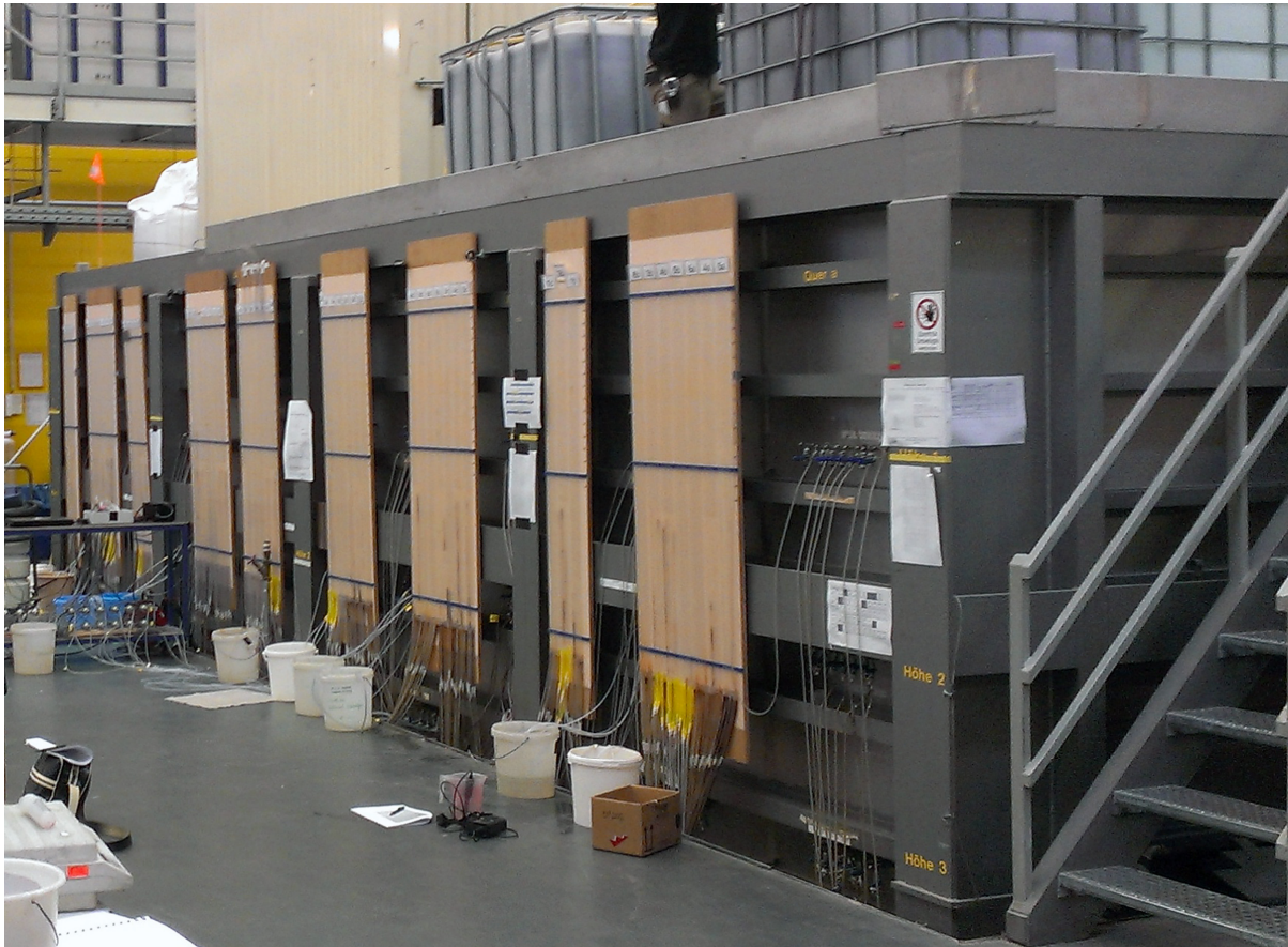
Figure 4.11: Photo of the upper half of the container at VEGAS, with the sampling ports (with tubes connected to them) on the side wall. The other part of the container and its sampling ports are accessible from the lower level of the facility. On top are the full tanks with the GNP suspension.
