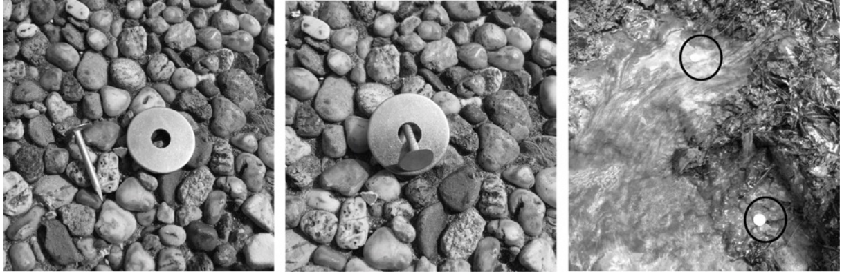
Fig. 2. Artificial substrate used for calcium carbonate precipitation measurements.
