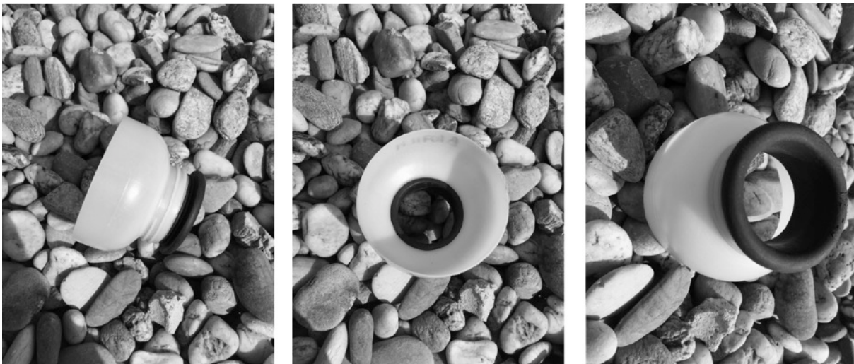
Fig. 4. 250 ml bottle modified with rubber lip for travertine microhabitat samplings. For fPOM and cPOM samples, the lip was removed and the bottle was used as sediment core (sampling depth = 2 cm).
