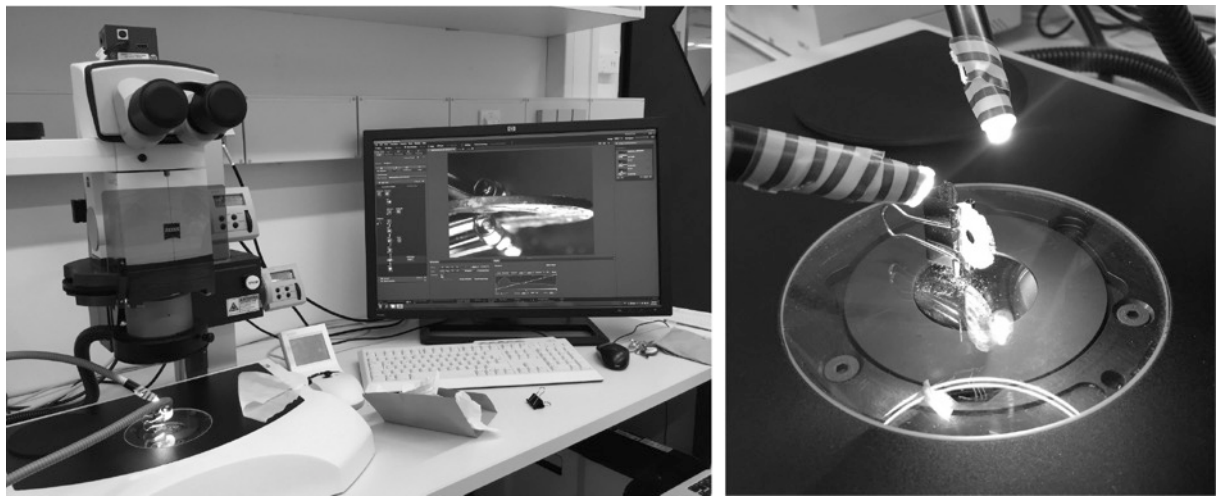
Fig. 3. Measurement of calcium carbonate precipitation. A binocular was used to measure the thickness of incrustation on field-exposed disks.
