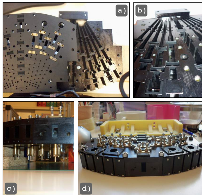
Figure A.1: Integrated Optics Assembly. (a) shows cover and base part of one optical plate. The Cover plate (to the left) is coated with a matt top coat whereas the base plate (to the right) is not. The influence of the matt layer on the reflectance of the material is clearly visible. Lenses and pinholes installed in the base plate (b) are adjusted using fine thread screws (d) pressing the elements against spring mounted pins (c).
