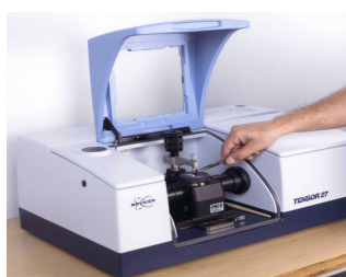
Figure 2.1: FT-IR Spectrometer - TENSOR 27 from Bruker Optics/Germany (35)
