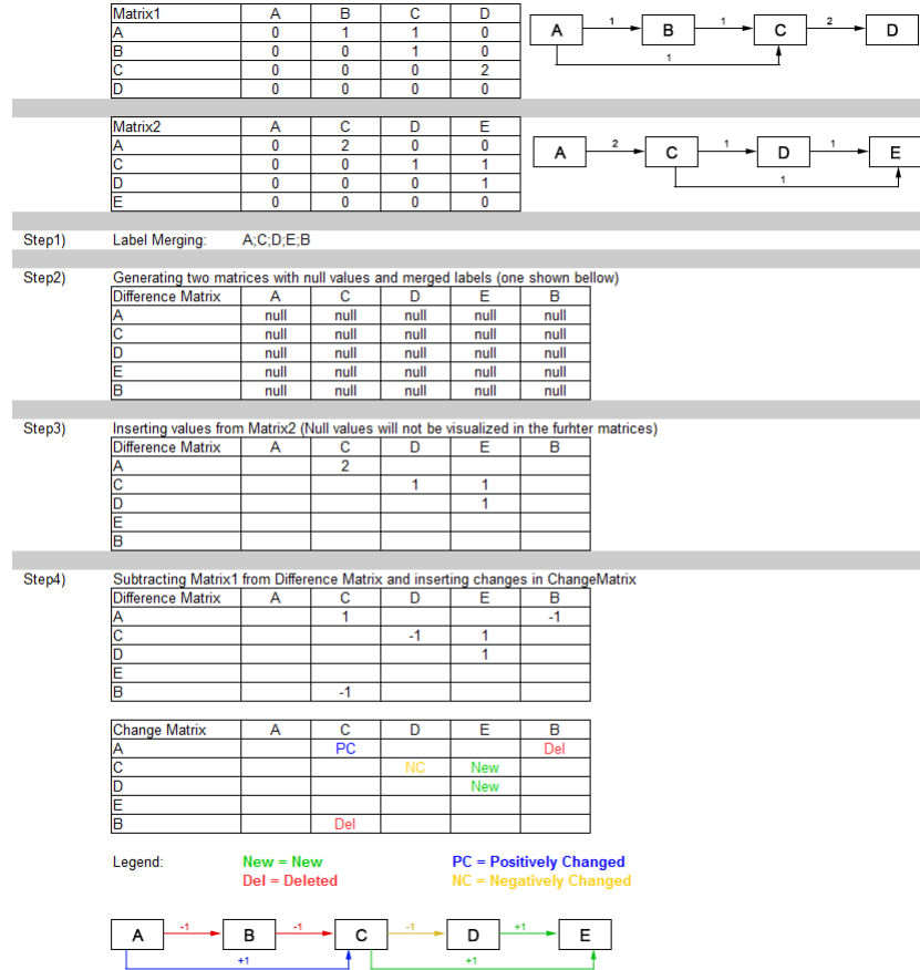
Figure 23: The input for the difference calculation are two matrices. On the right of the matrices the corresponding graph is visualized. Those two matrices are used as input for the difference calculation which is divided in four steps and results in a difference and change matrix. The result is also visualized as color coded graph.
