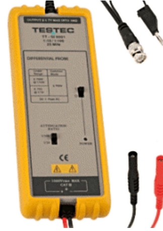
Figure 3.13: A differential probe with BNC-plug and banana-plug is used to convert the high voltage signal from the PVAS output to a low voltage signal for the DAQ-box. It provides attenuation factors of 10 and 100.
