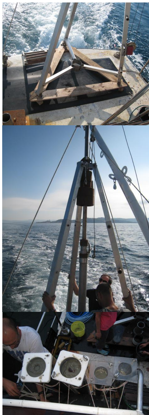
Fig. 3: Piston corer with hammer action. Tripod for stabilization on seafloor during coring operation (A), mobile weights hammering the cylinder into the seafloor (B), extracted sediment in upright position ready for slicing (C).
