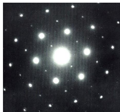
Figure 48 Example of an electron diffraction pattern of a hexagonal cell [49]
