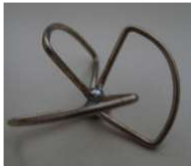
Figure 22: Clover leaf right hand polarized 5.8 GHz video antenna, usually used with a (RP-)SMA connector, working as a remote antenna on the UAV
