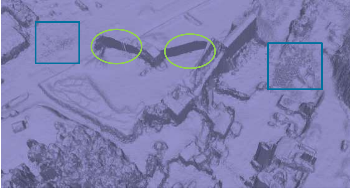
Figure 45: Issues: note rough ground (blue boxes), conveyor belt with filled headspace (green circles)
