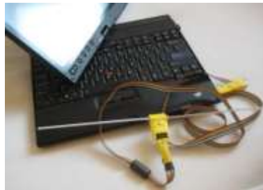
Figure 20: Typical ground station, a standard laptop with UHF serial modem; note the long cable to avoid interference from the USB bus to the modem
