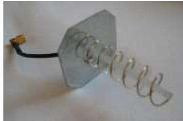
Figure 21: Helical right hand polarized 5.8 GHz video antenna, used for better reception at ground station
