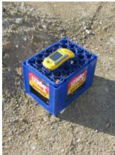
Figure 15: Base station for differential correction; note that for increased accuracy the dome of the GNSS antenna was placed level with an additional cardboard box (not visible in photo), crate was used to increase reception
