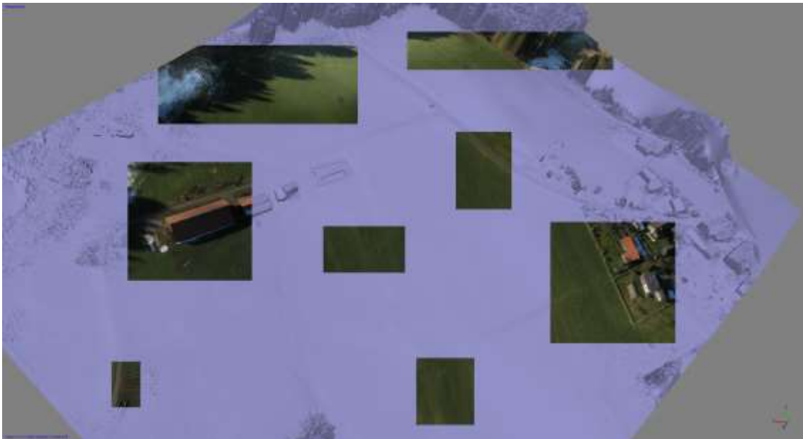
Figure 34: First aerial photos, revisited with Photocan; shaded model with partial overlays of projected photos
