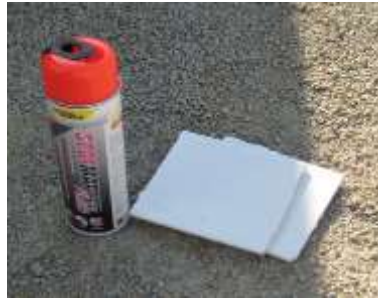
Figure 9: Used spray-paint; for best results use old discarded tiles for best reflectance and visibility
