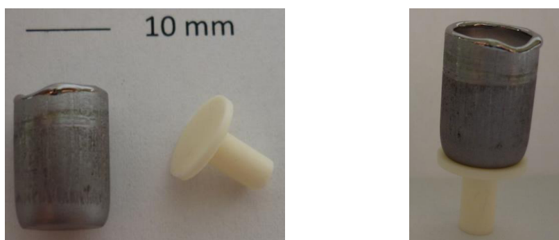
Fig. 15: Ta crucibles used for DTA measurements
