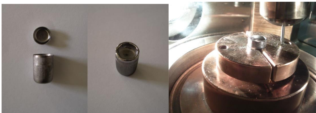
Fig. 13: Ta crucible were enclosed by arc welding
