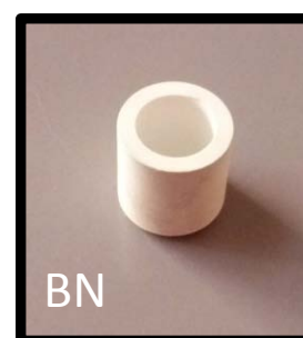
Fig. 25, Boron nitride crucible for sample preparation.
