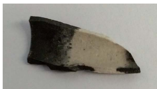
Fig. 24, A part of the magnesia crucibles purchased from Morgan Refractories; the black material which penetrated the crucible is antimony, which settled in the pores of the material.
