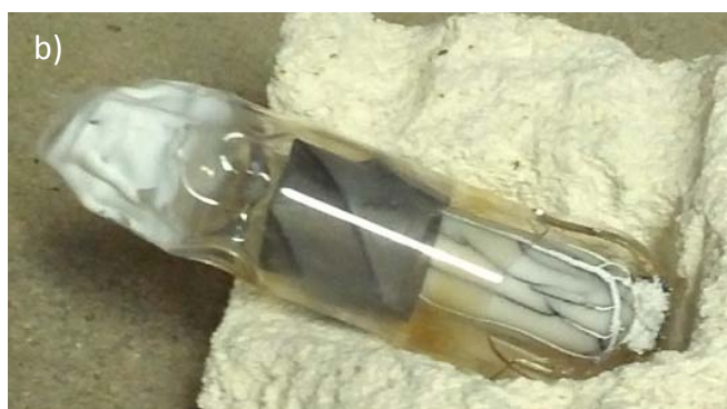
Fig 22a, mixed oxide layer formed on an alumina crucible due to reaction with lithium; b, lithium diffused through tiny cracks in the crucible and reacted with the silica tube. After the silica tube broke, the lithium immediately oxidized (white powder at the bottom).
