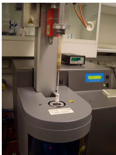
Figure 24: DTA-instrument Setaram Setsys Evolution TGA & DTA 2400
