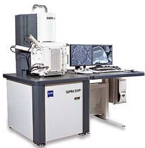
Figure 21: Zeiss Supra 55VP SEM/EPMA
