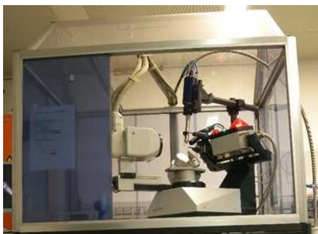
Figure 23: Single crystal-XRD Bruker Nonius KappaCCD FR590
