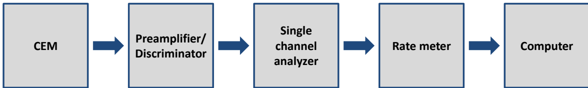
Figure 4.9: The output pulse of the CEM was processed using a preamplifier/discriminator, a single channel analyzer, and a rate meter connected to a computer system.
