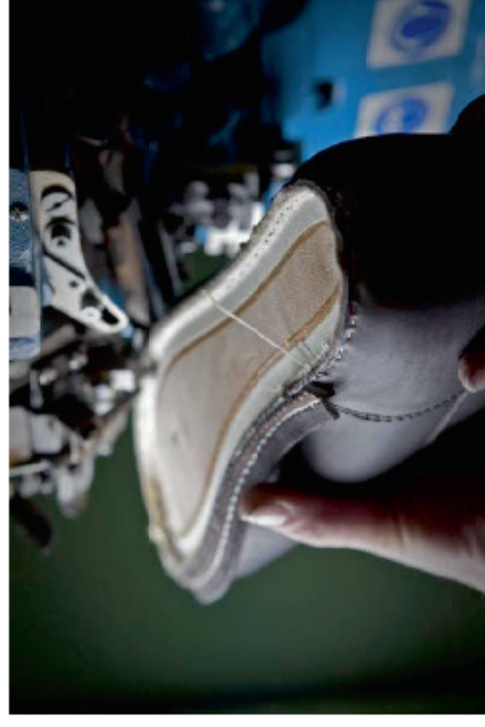
Step 1: The upper leather and inner sole are sewn together with a continuous leather strip.
