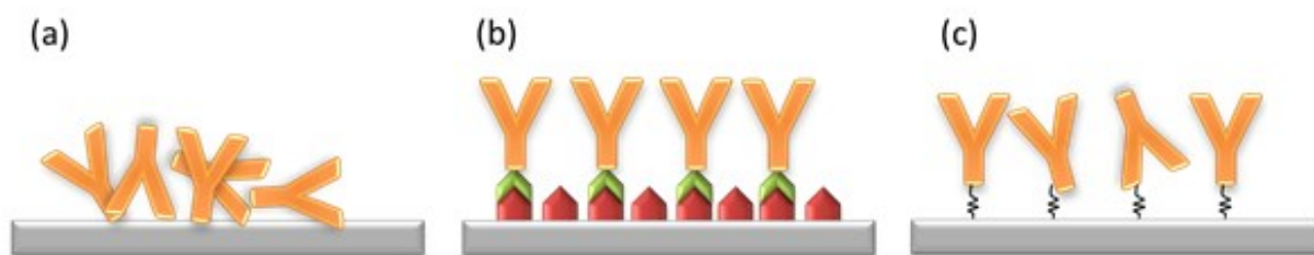
Figure 12: Schematic depiction of the various immobilization strategies: (a) physical, (b) bioaffinity and (c) covalent attachment
