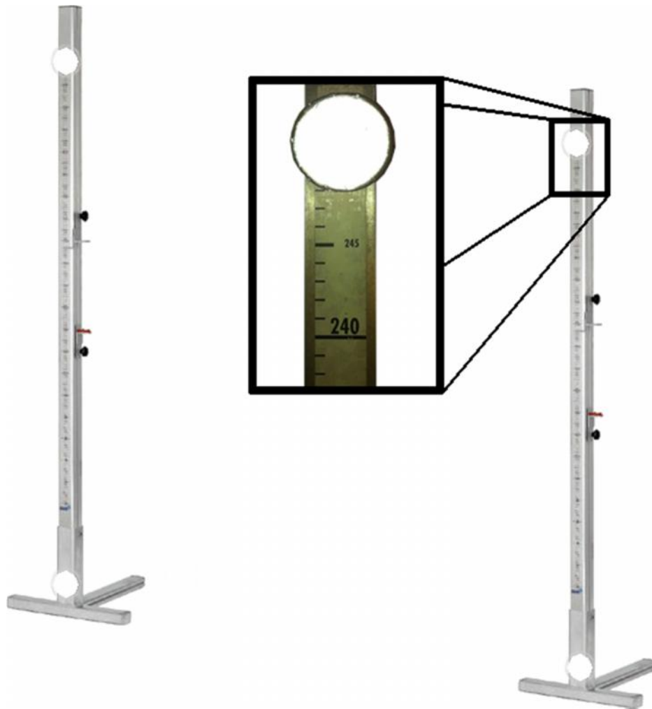
Figure 9: Calibration markers on the grid
