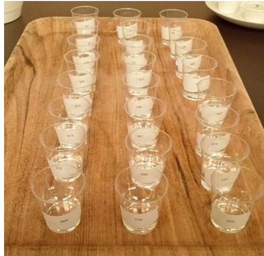
Figure 8: 24 samples, each row containing one salt and two water samples
