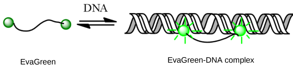
Figure 7: Intercalation of the dsDNA binding dye EvaGreen, from [58]
