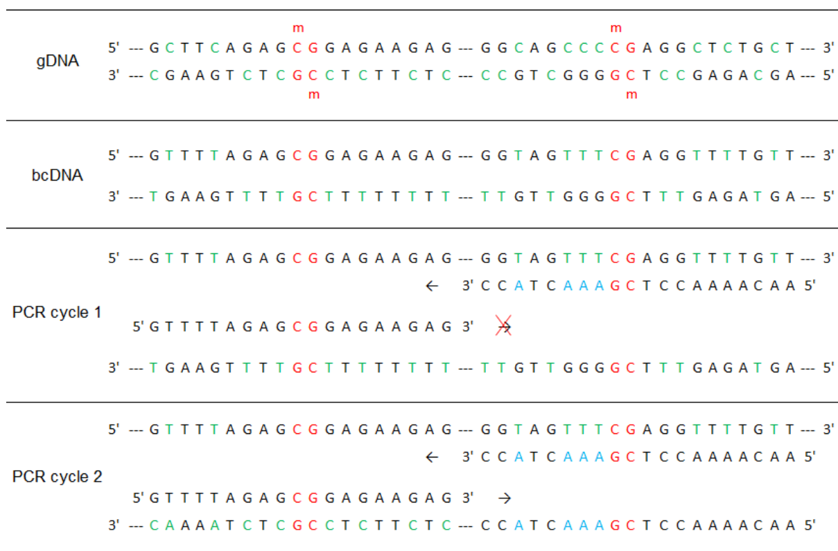
Figure 21: Schematic illustration of primer annealing in the first two PCR cycles
