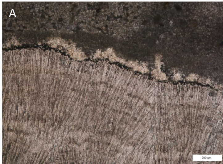
Fig. 12 A: Bundles of aragonite needles pointing towards the center of the pipe rimmed by pyrite crystals (SMFSR). B: Co-occurrence of yellow (YA) and clear (CA) aragonites at the boundary to brownish calcite (BC) (SR4).
