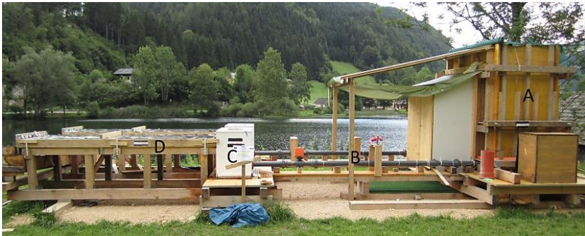
Picture 1: Experimental setup. From right to left: header tank (A) linked by two pipes (B) with the white smaller tanks (C) and then with flume panels (D)
