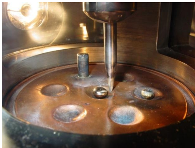
Figure 14. Water-cooled copper plate, serves as anode. Under an argon atmosphere of 0.5 bar, using zirconium (in the centered position) as a getter material, the alloy is melted.
