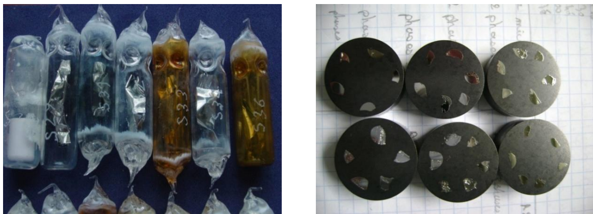
Figure 15. Sealed and evacuated quartz glass tubes with (quaternary) ingots wrapped in Mo-foil and embedded samples.
