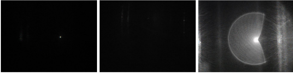
Figure 8.1: Pictures from three cameras. Pictures are taken simultaneously from three cameras with overlapping field of view. The first two pictures show the space close to cavity mirrors, which is not possible to observe on the third camera. The image of the particle in the third picture is clearly cut by the retaining ring holding the mirror. The same particle is also seen in the first picture.
