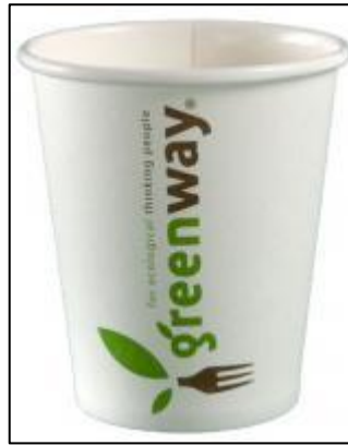
Figure 3. Bio-degradable paper cup without plastic coating, used in the experiment
