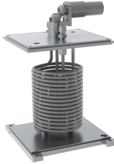
Figure 4.17: The water bath heater with a tube spiral, a stirrer and two heating cartridges. The side walls are not shown. The filling volume of the water bath heater is about 4l.
