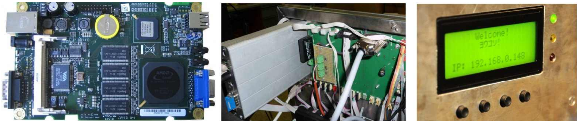
Figure 4.22: Alix3d3 single board computer, expansion board and display.
