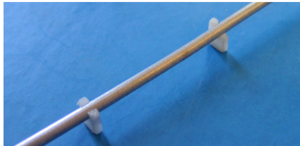
Figure 5.9: One part spring-clamp-v1 prototypes, assembled with an evaporation tube.
