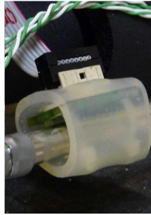
Figure 4.19: Digital temperature sensor DS620 assembled on a tube (6mm outer diameter).
