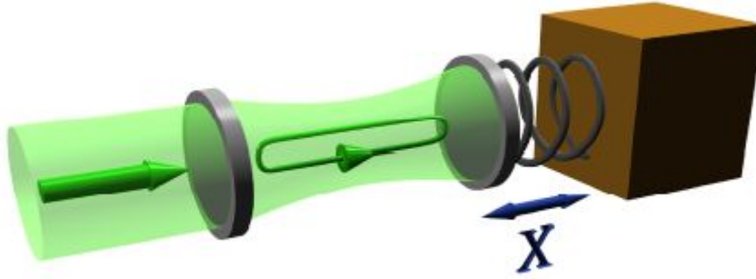
Figure 2: basic optomechanical setup(from [20])
