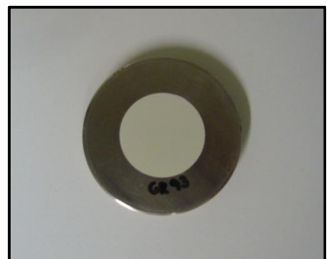
Figure 6 Pressed powder in sample holder
