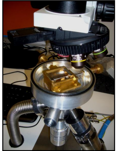
Figure 10 Sample in vacuum chamber (open)
