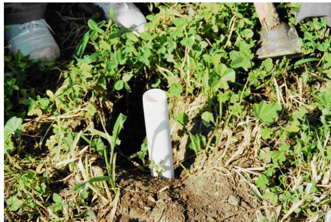
Figure 2.15.: Mineralogical sampling using a 1m long, hollow plastic tube with caps on both ends. Pipes were pushed into the ground using hammers, then pulled out, and closed for further transportation.
