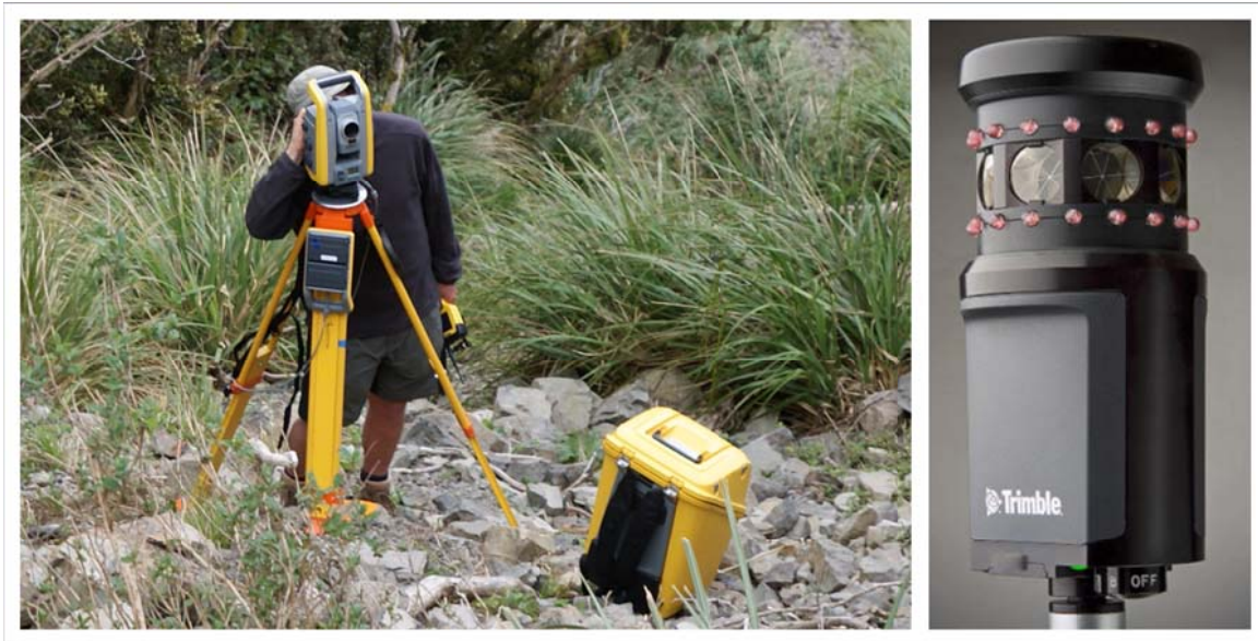
Figure 4.2: Left picture: Installed Trimble S6 DR300+ robotic total station at work. The data logger in the scientists left hand is remotely connected to the station. Right picture: Highly reflecteable 360° prism used as physical target for point measurent. (own picture 2011 and flickr picture database 2012)
