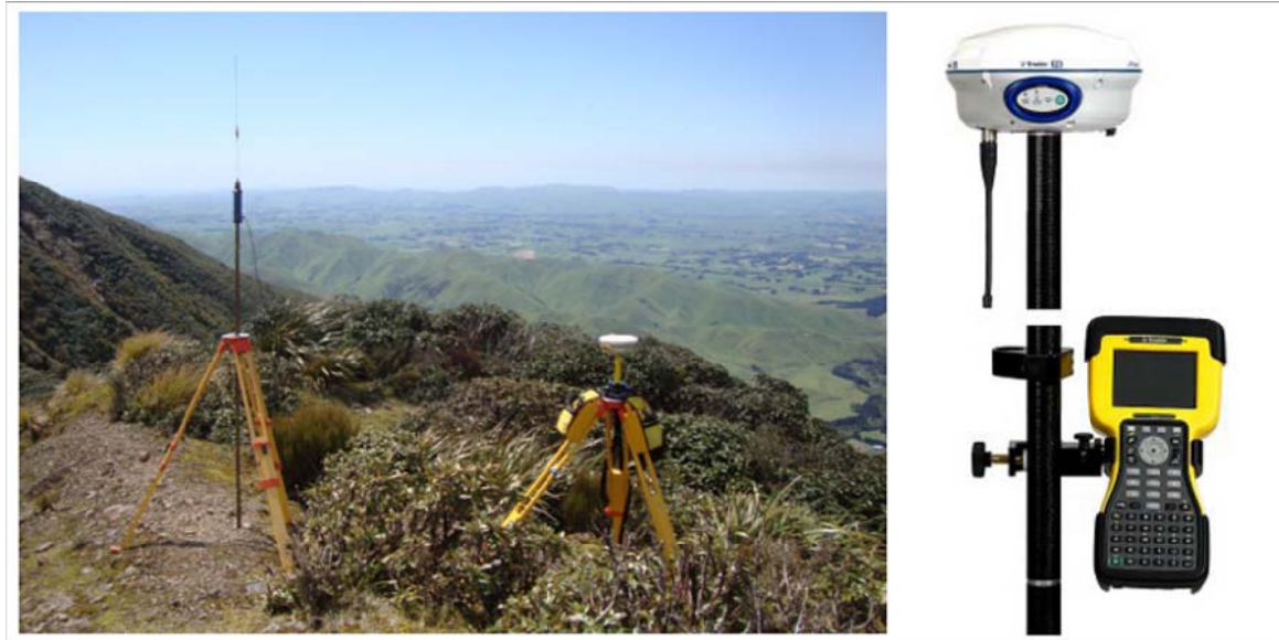
Figure 4.1: Left picture: Trimble R8 base station with radio device on a long metal pole on the left side, set up at the ridge above Tamaki West Catchment. Right picture: Trimble rover consisting of the antenna (white) and the data logger (yellow) fixed on a 2m carbon fiber pole including the spirit level on the small black triangle.(own picture 2011 and online rataling site azannunci 2012)
