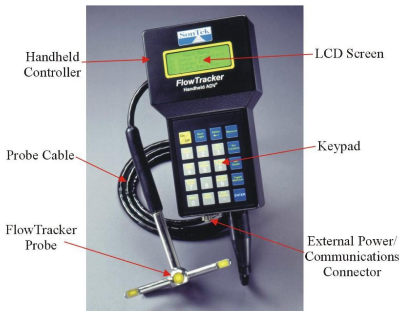
Figure 12 Flow Tracker with 2D Probe (S: User’s manual, 2009, p.1)
